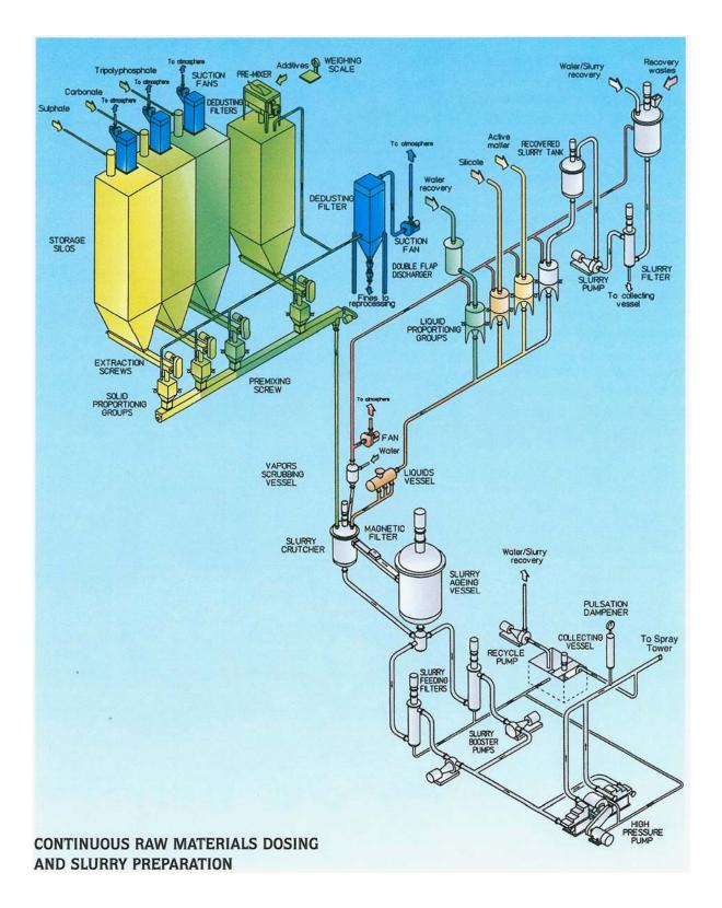
The concentrated, viscous slurry, is fed through magnetic traps followed by special self cleaning filters designed to remove any possible solid particles which could damage or clog the pumps and the spray nozzles.
