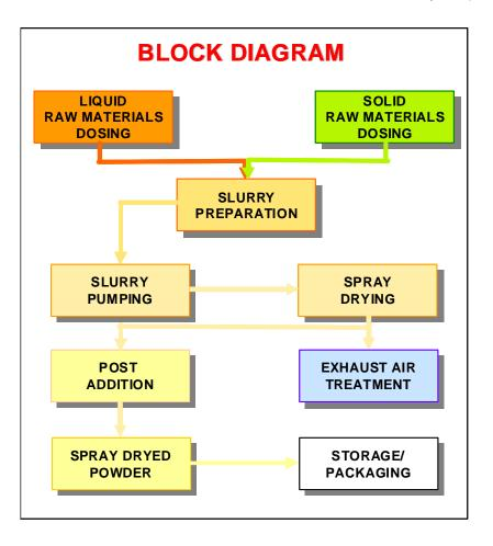
In the Continuous Slurry Preparation system, solid and liquid ingredients are individually and automatically dosed by means of electronic scales operating over variable weighing cycles, in accordance to product recipes and plant production capacity. The proportioned ingredients are continuously fed to the slurry crutcher.
